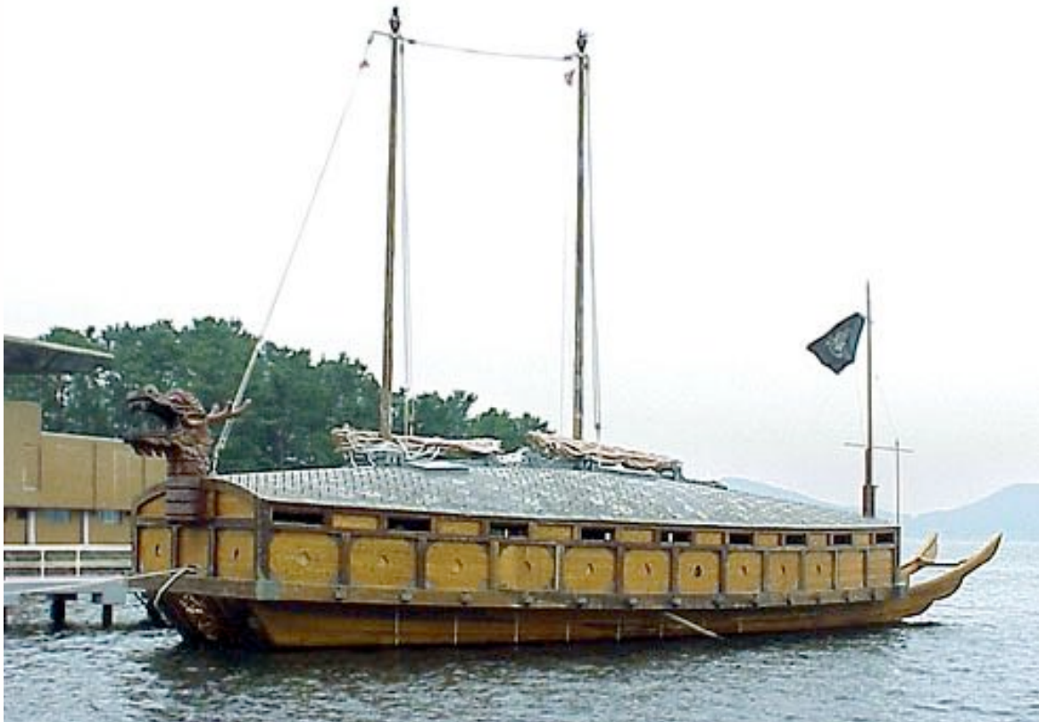
A reconstructed full-size replica of a Turtle Ship, the usual length being 30 to 37 metres. Propulsion, 80 oarsmen with a complement of 50 soldiers. Armament, 26 canons.
