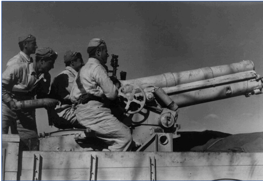
Figure 4: The Italian Ariete division utilised truck mounted four-inch naval guns (Batteries Milmart from the Naval Auxiliary Service) in the defence of the Bir el Gubi positions.
